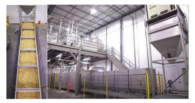
Napasol Pasteurisation line of 6 bins showing full bins from the top (left) and bins lined up on the loading platform ready to enter the pasteuriser. Photos courtesy of Poindexter Nut Company. CA, USA
